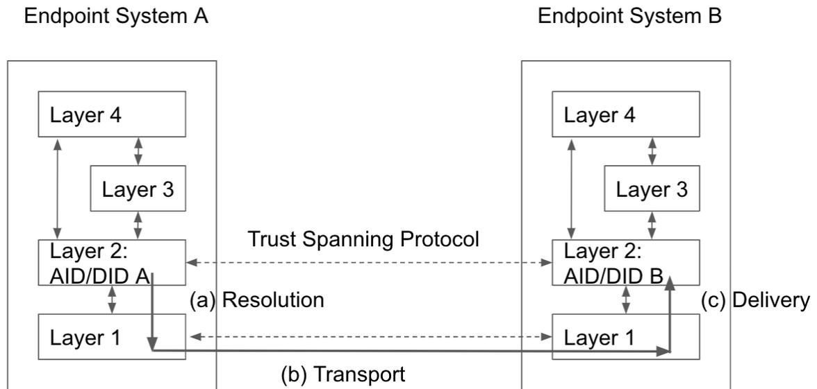
**Figure 8: Overview of the ToIP Spanning Protocol**
